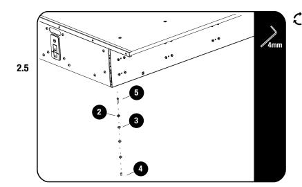
Stack three M8 x 19 x 3 Flat Washers (Item 3) on top of the Rivnuts to compensate for the carpet thickness. Carfully place the Drawer System on top of the stacked washers. Fasten the Drawer System in place using M6 x 25 Countersunk Cup Screws and M10 Flat Washers (Item 2 & 5).
