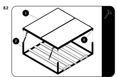
Flip Sub-assembly 6 (Item 1), so the remaining stems (D) on the corners are facing downwards.
