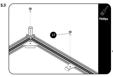
Using a No.8 x 16 Pan Self-tapping Screw (Item 17), fasten each bracket to the deck. This will attach the Deck to the frame.
