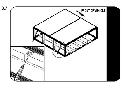
Position the D-Rings so that the Turnbuckles will pull outward to prevent the Drawer System from moving after it has been secured.
