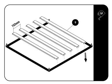
Place the five Bottom Supports (Item 9) over the Extrusions loaded in Step 3.1.
