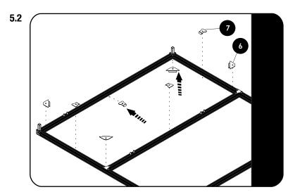
Place the Corner Brackets (Item 6) in each corner by slotting them into the inner slot of the Extrusion, as indicated by the arrow in Fig A and Fig 5.2, and align the holes with the pilot holes on the Deck.
