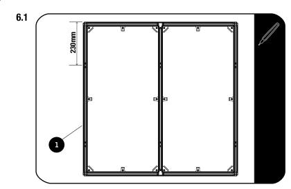
Using Sub-assembly 4 (Item 1) from the previous step, measure 230mm from each side, as shown and mark each Extrusion with a Marking Pen.
