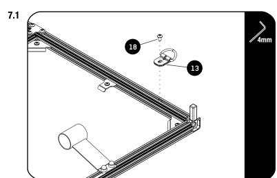
Loosely assemble the D-Rings (Item 13) using the two outer M6 Thin Nuts (Item 21) that was loaded in Step 2.1 and a M6 x 10 Button Head Bolt (Item 18).
