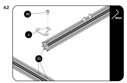
Loosely assemble the Joiner Plates (Item 4) on each end of the Extrusion (Item 1) using the first and last M6 Thin Nuts (Item 21), loaded in Step 4.1 and M6 x 8 Button Head Bolts (Item 20).
