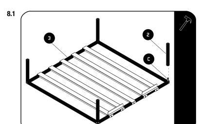
On a flat surface, place Sub-assembly 2 (Item 3) so the remaining stems on the corners are facing upward.
