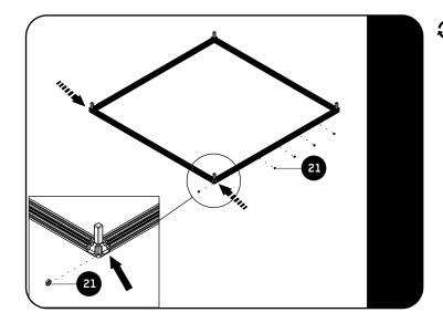
Starting with the Bottom Frame, as assembled in Step 2, load five M6 Thin Nuts (Item 21) into one of the 915mm Long Extrusions, using the slot on the outside of the Corner and Extrusion.
