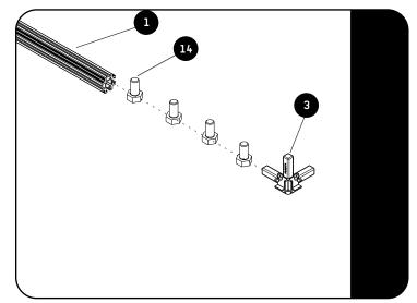
Load four M6 x 12 Hex Bolts (Item 14) into an Extrusion (Item 1), as shown in Fig. 2.1.
