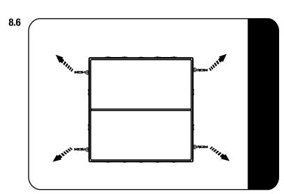
Place the Drawer System in the vehicle and center it. Make sure the Turnbuckles will be pulling outward to the existing mounting points in the vehicle to prevent it from moving after it has been secured.
