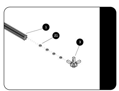
Load four M6 Thin Nuts (Item 21) into each of the two remaining Extrusions (Item 1), as shown in Fig. 2.2. Place these opposite each other.
