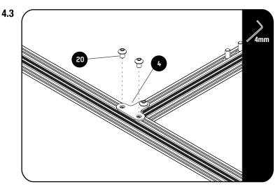
Align the middle two M6 Thin Nuts (Item 21) of the four that were loaded in Step 2.2 with the holes in each Joiner Plate (Item 4). Do this for both sides.
