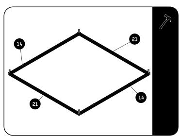
Use the Rubber Mallet to securely fit the corners so they are flush against each Extrusion. This will be the Top Frame.
