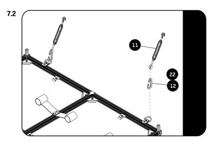
Hook the Carabiner - Large or Small, depending on the vehicle's mounting points - and Turn Buckle (Items 11 & 12 or 22) onto the D-Rings for use when installing in the vehicle.
