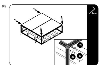
Loosely assemble the Corner Gusset (Item 23) using two M6 Thin Nuts (Item 21) and two M6 x 8 Button Head Bolts (Item 20). Load the whole assembly into the front and back corners, as shown.
