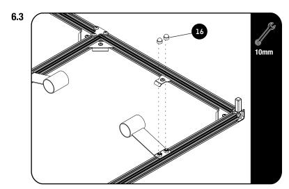
Adjust Springs if necessary and tighten all fasteners.
