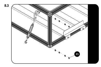
Load four M6 Thin Nuts (Item 21) into the outer T-Slot on the bottom and top Extrusions parallel to the Bottom Supports, as shown in Fig 8.3.
