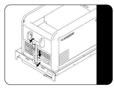
Feed the latch end of the Quick Release Latching Strap through the handle of the fridge, then through the tie down points on the fridge slide.
