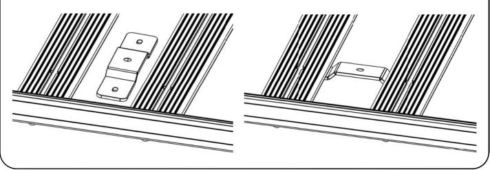
(E) Working from underneath the Rack, line up the Hex Bolts from Step 2B with the machined slots in the Rack as indicated. Lift the Bracket, inserting the Hex Bolts into the machined slots. Slide the Bracket Assembly into position (Left to right) making sure the Hex Bolts remain in the Racks "U" channel.
