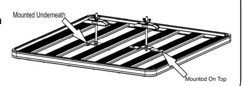
( **B** ) Referring to the Exploded View on Page 2 and the fitment chosen (On top or underneath), loosely assemble Items 8-10 to either side of the Mounting Bracket (Item 7) as shown.
