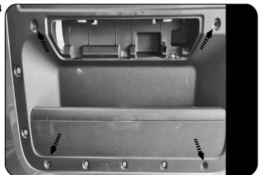
Remove the OEM Bolts as shown.
