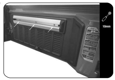
If your vehicle has the cargo Rail fitted, remove it by loosening and removing the three bolts shown.
