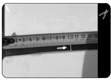
Looking at the front of the ditch molding, measure 100mm backward from the front and make a mark
