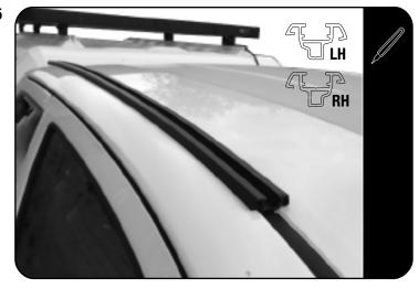
Place the LH Track into the LH ditch and RH Track into the RH ditch. Ensuring they are fully seated.
