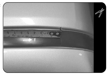
C) Looking at the rear of the ditch molding, measure 40mm forward from the joint line and make a mark.
