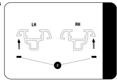
Fit the Foam Strips (Item 2) by removing the backing tape and apply them to the outside profile edge of each of the Tracks as shown in 2.3.
