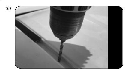
Before drilling the holes in the roof, you need to do a bit of prep. Take both the 3mm and 6 mm drill bits. Using a suitable tape, wrap a band of tape around the drill bit to act as a guide / stopper to prepent you from drilling. ⚠ / stopper to prevent you from drilling too deep as there are airbags located
