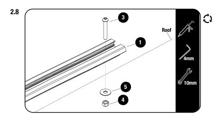
Place sealant in and around each of the holes drilled.
