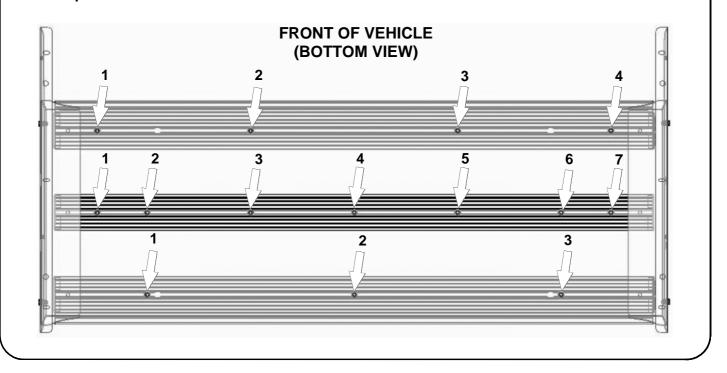
(**B**) Working underneath the Slats, position the Rear Top Hat (Item 13 - the longer one) between the back two slats. Lift the Top Hat into position lining up the holes in the Top Hat with the Half Nuts inserted in Step 4A. Hand tighten the Top Hat to the Slats using the M8 x12 Button Head Bolts and M8 Schnorr Washers (item 15 & 16) Supplied.
