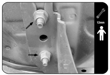
Start by opening and placing a suitable support under the front of the hood to help support it while you remove the bolts.
