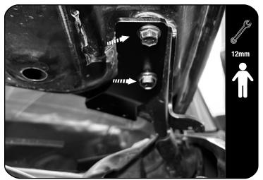
Start by opening and placing a suitable support under the front of the hood to help support it while you remove the bolts.
