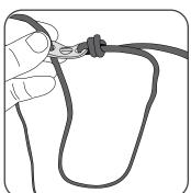
In the opposite end of the Guy Line, tie a loop. A figure 8 knot works well.
